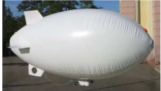
Fig. 1. This images shows the completely build blimp with a length of 1.8 m and a diameter of 0.8 m.
