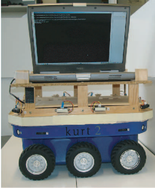
Fig. 3. The robot KURT-2, with the controlling notebook on top, and the infrared distance sensors.
