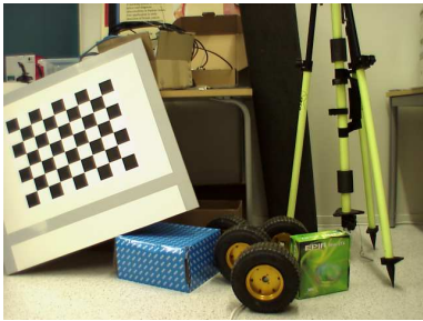
Fig. 4. Calibration board used to determine the calibration parameters of the camera, with a chess board texture and reflective tape (gray border) to locate the board using remission / intensity values from the laser scanner.
