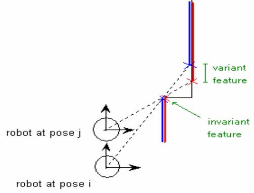
Fig. 1. Lines in black represent the environment, blue and red lines are the acquired scans from pose i and j, respectively. Upper feature is varying with respect to robot's displacement, but the other feature is an invariant one.
