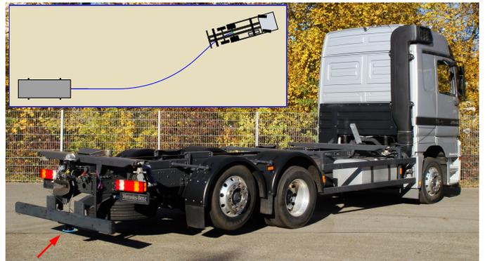
Fig. 1: Test vehicle with rear 2D laser range scanner approaching a target object on a planned trajectory.
