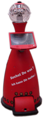
Fig. 1: Robot platform SCITOS A5 by MetraLabs GmbH (Fig. 1), which features a quite accurate odometry.
